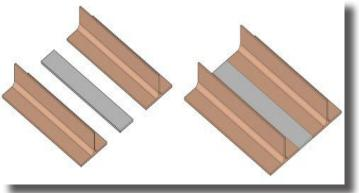
Figure 10 (above) Schematic of rolled channels and spacing plates. (Below) Example of a fully forged ISP.
