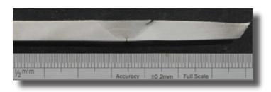
Figure 7. A metallographic section through a deliberately defective FSW in 6mm thick DH36 steel. The failure site is in the parent metal to the right hand side of the sample.
