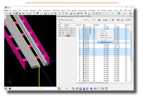
Figure 5: Functionality to visualize 3D model of cables on design review task. 3D model of cables routed in a tray segment.
