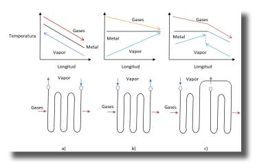
Figure 2. Temperature variation of streams and exchange surface according to counterflow (a), parallel (b) and mixed (c) configurations.
