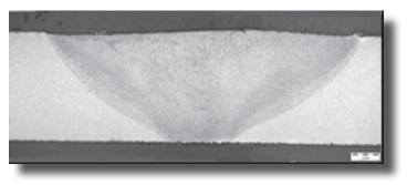
Figure 2. A metallographic section through a single pass FSW in 6mm thick DH36 steel.
