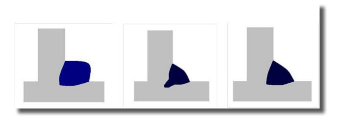
Figure: effect of CO2, argon and Ar/CO2 mixtures on the penetration profile for MAG welding.
