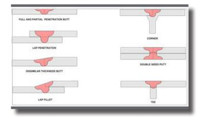
Figure 3. Joint geometries most easily achieved in FSW.
