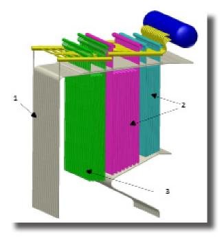
Figure 1.- Heat exchangers in a steam generator with predominance of transfer by radiation (1), convection (2), convection-radiation (3) [1].
