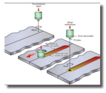
*Figure 1. The general principle of friction stir welding.*
