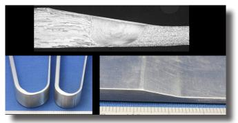
Figure 5 Example of a joint made between 4mm and 2 mm thick AA6082 sheet. The macrograph (upper) shows the weld to be defect free and the root and face bend test samples (lower left) attest to its mechanical integrity. The smooth transition between the two different thicknesses of material is shown lower right.
