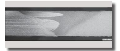
Figure 9. Metallographic section through a weld made between 8mm thick S355 carbon steel and S32205 Duplex stainless steel.
