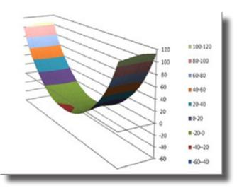
Figure 8a (above) showing the distortion measured in a SAW and 8b (below) showing the distortion in a FSW, both in 6mm thick DH36 steel. (Data courtesy of BAE Surface Fleet)
