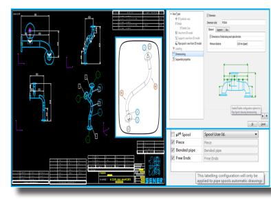
Figure 4: New area in drawings template allows to configure dimensions needed in that area of automatic drawing.
