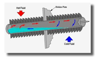
Figure 8. Thermosyphon tube where the circulation of the steam generated on the hot side, towards the cold side is represented. Once condensed, it returns by gravity to the hot side [6].
