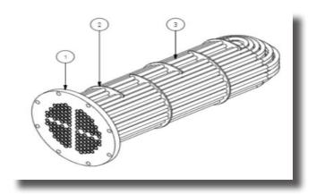
Figure 7.- Tubular U-shaped bundle with triangular arrangement showing 1-plate; 2-deflector or baffle; 3-tube bundle.
