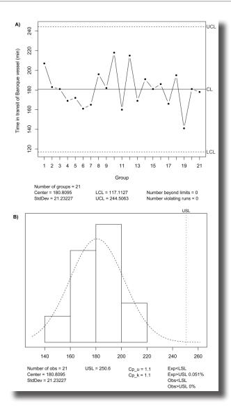
Figure 5. A) Control chart for transit time using the last 21 transits of the vessel Baroque. B) Histogram and density function assuming normal distribution of transit time, upper specification limit (USL) and capacity analysis.
