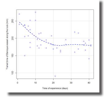
Figure 4. Relation between the days of experience of the pilots and the times of transit in the Canal with the Baroque data sample. Fitting a non-parametric Loess regression model.
