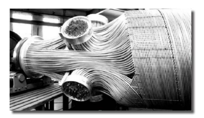
Figure 9. Linde spiral tube heat exchanger for LNG reliquefaction [7].
