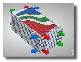
Figure 5.- Corrugated plate heat exchanger, compact, recuperative, with exchange between three streams [4].
