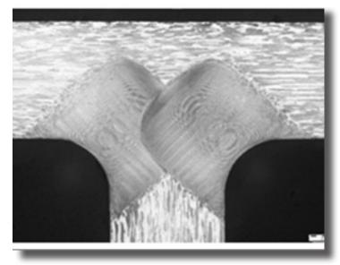
Figure 4. Metallographic section through a radiused corner fillet weld made by two FSW passes in 8mm thick AA6082.
