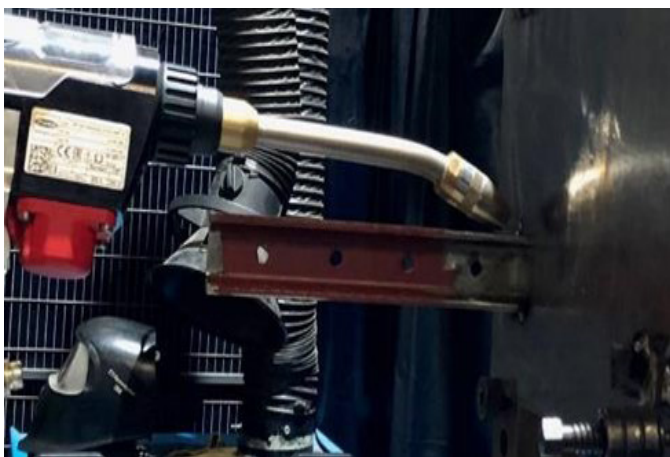
Figura 14. GMAW parameterization of a typology of support in AIMEN laboratories.
