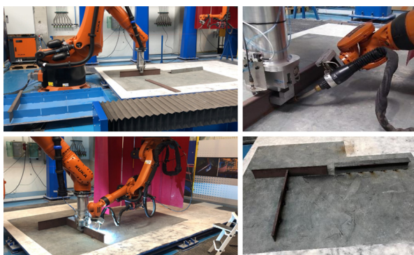
Figure 11. Different steps in the manufacturing sequence of the demonstrator developed at AIMEN's facilities.
